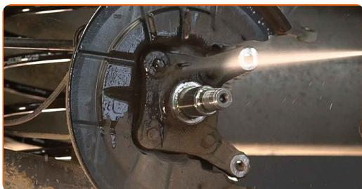
**20** Install the new wheel hub with a bearing.
