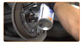
14 Install the new wheel hub with a bearing.
