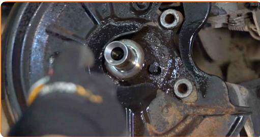
21 Install the new wheel hub with a bearing.
