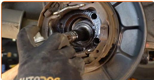
**22** Install the new wheel hub with a bearing.
