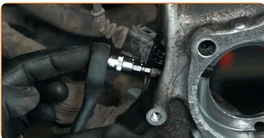
**43** Install the new wheel hub with a bearing.
